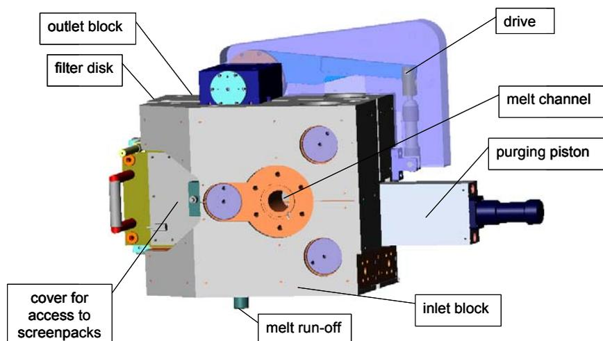
Fig. 6: RSF*genius* filtration system
