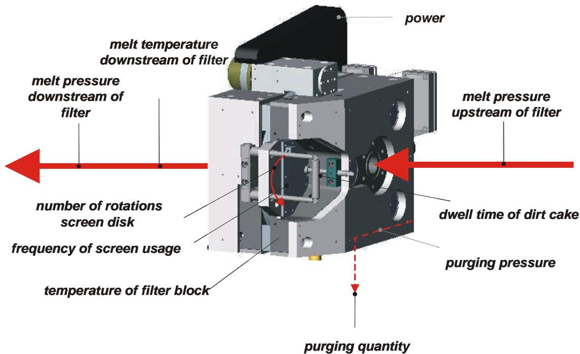
**Fig. 8: Controlling Principle of the RSFgenius**
