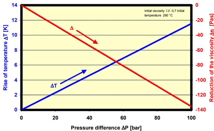
Fig.5: Variations in the melt temperature and viscosity due to pressure variations during the filtration of PET
