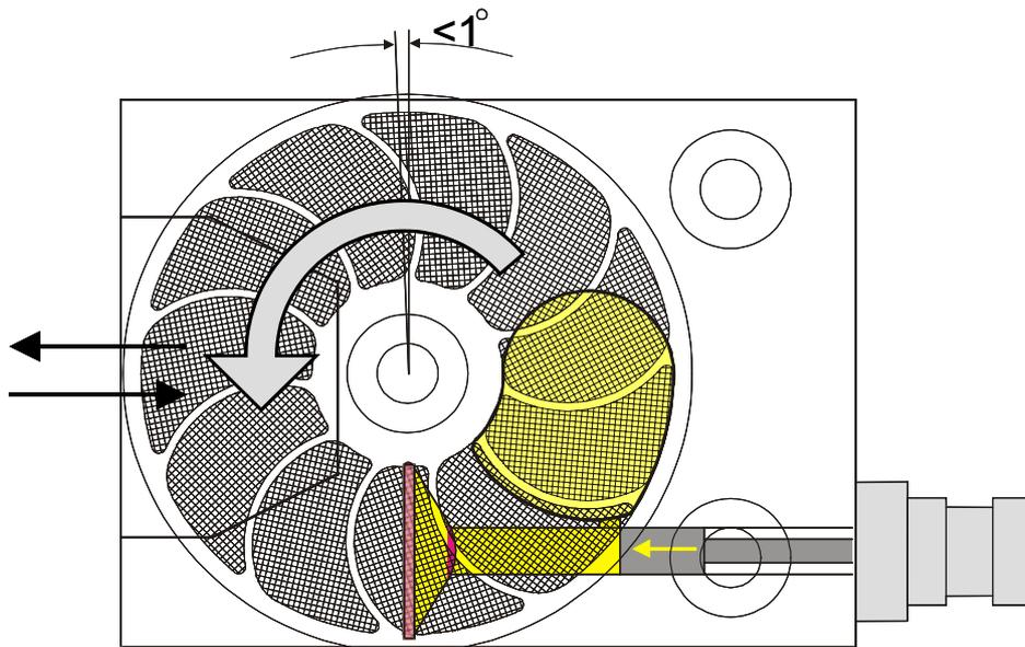
**Fig. 7: Operation of the RSF*genius* Filtration System**
