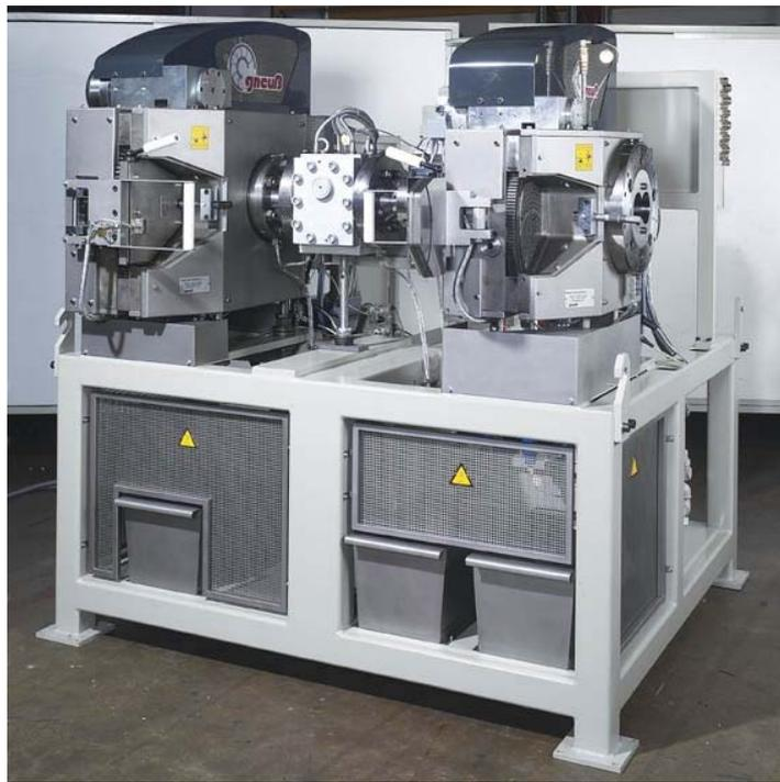
Fig. 9: Tandem Filtration System for a PET sheet line. Throughput rate: 1.200 kg/h.
