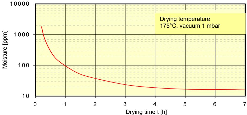
**Fig. 1: Drying curve of PET pellets with an edge length of 2,6 mm at a temperature of 175°C in a vacuum (1 mbar).**
