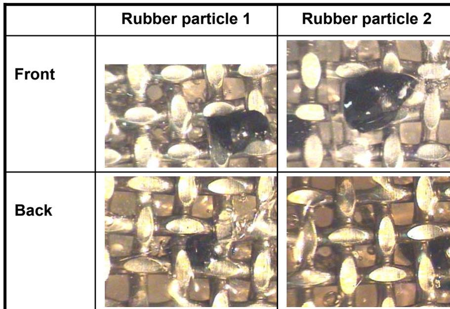
Fig. 4: Adhesion of rubber in the filter screen (filter fineness 200  $\mu\text{m}$ ,  $\Delta p$  pressure 100 bar)
