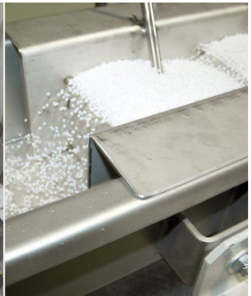
Crystallization conveyor for recycling applications
