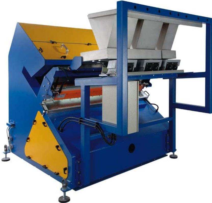
Additionally, S&S offers the PETMAG metal separation system, capable of detecting contaminants from 0.6mm in size – even if the metal is bonded or incorporated in the plastic. The system uses compressed air from a bank of ejection nozzles to remove the metal contaminants from the rest of the material. Capacity ranges from 500 kg/hour to 4 t/hour.
