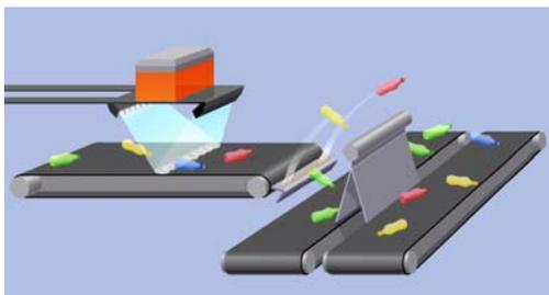
TiTech's innovative sorting technology makes it possible to fully automate separation of recyclable materials. The input stream is analyzed by a fast-scanning sensor installed over a conveyor belt. It rapidly identifies materials, shapes, textures and colours as well as the object position. TiTech blows the defined sorting fraction onto a second transport system
