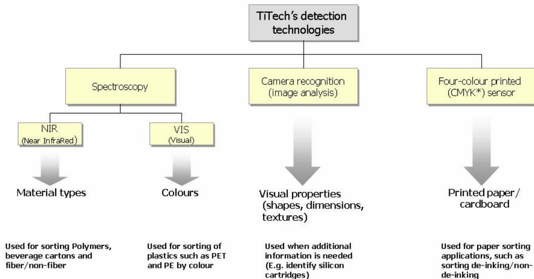
The system's high precision and high speed makes it possible to sort an input stream up to 10 t/h with high performance. Our systems create high amounts of labour savings and increase the sorting quality at the same time. Typical efficiency and purity rates are in the 90 – 98% range.
