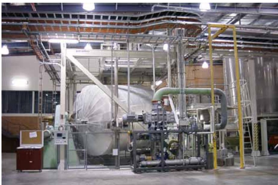
Figure 7. OHL vacuum vessel used in Phoenix process in Australia at Visy Prestons plant.
