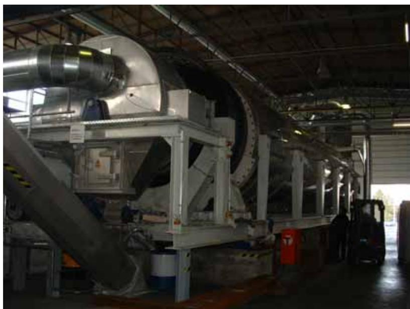
Figure 6 Tubular reactor for treating flake and caustic mixture.
