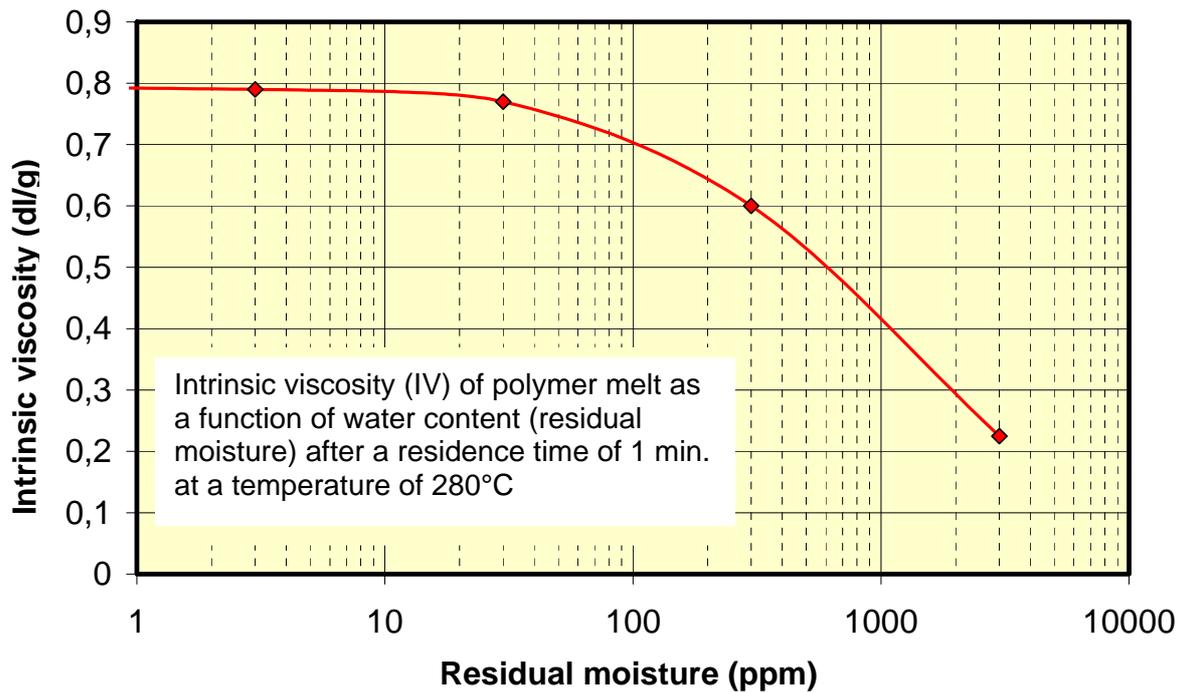
**Illustration 1: Polyester degradation by hydrolysis - IV of polymer melt as function of water content (at 280°C, residence time 1 min)**
