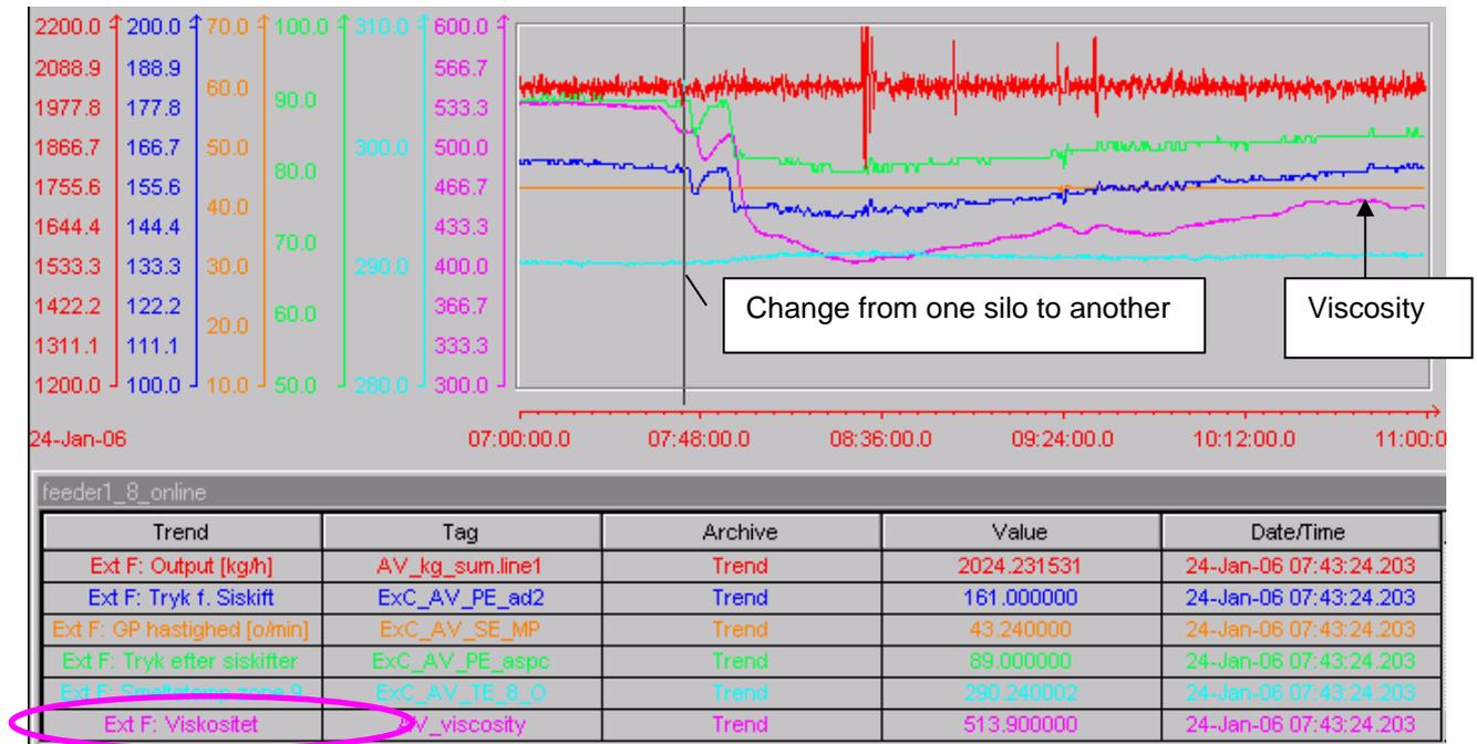
**Illustration 6: The viscosity trend shows a material change from one dryer silo to another. The viscosity drops and after a few hours returns to the original level.**
