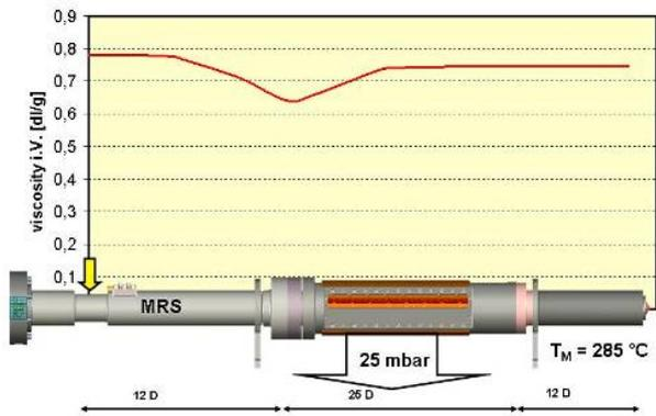
Fig.6: Viscosity when processing PET –Bottle Flakes
