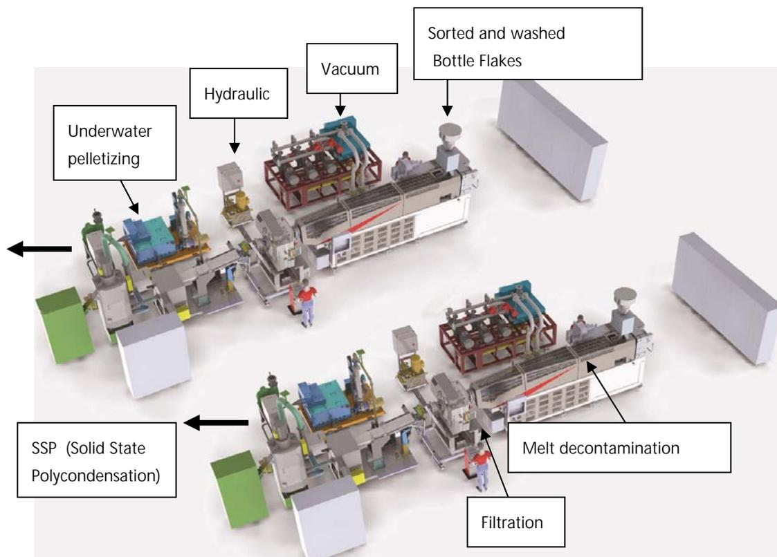
Fig.11: Arrangement drawing of extrusion equipment
