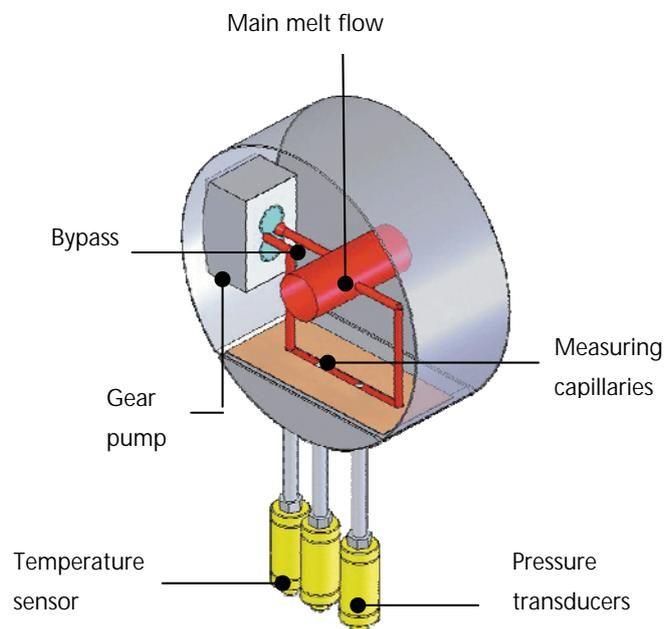
Fig.8: Online Viscometer VIS –technical layout
