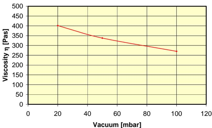
Fig.7: Correlation between viscosity and vacuum applied
