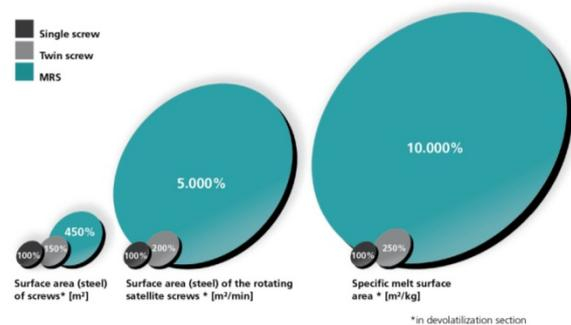
Fig.5: Comparison of different extrusion concepts
