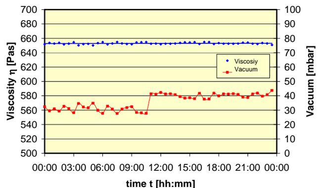
Fig.9: Viscosity in relation to residual moisture variations
