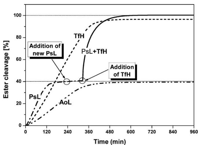
Fig. 5. Degradation of poly(butylene adipate) films with different hydrolases at 40 °C in 0.9 M NaCl solution. AoL: Lipase from *Aspergillus oryzae*, PsL: lipase from *Pseudomonas sp.*, TfH: hydrolase from *Thermobifida fusca* [19].
