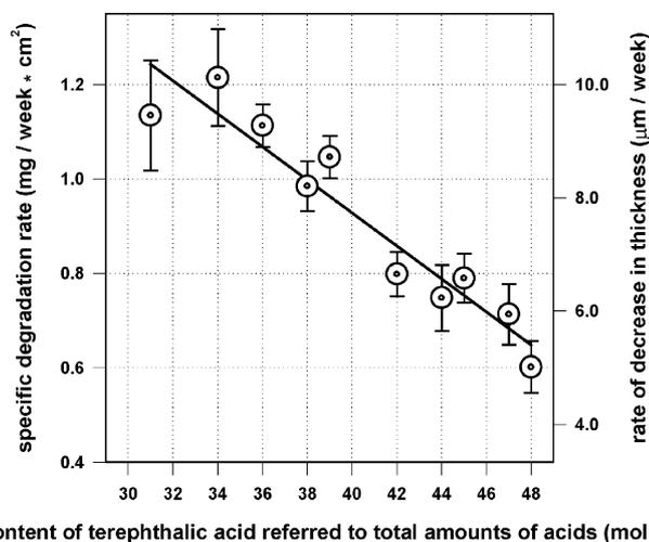
Fig. 3. Decrease in degradation rate (monitored as weight loss) of films of aliphatic-aromatic copolyesters (BTA, copolyesters composed from adipic acid, terephthalic acid and 1,4-butanediol). Incubation of films on a mineral medium agar plate inoculated with a pre-screened microbial culture from compost at 60 °C. Test duration 6 weeks [14].
