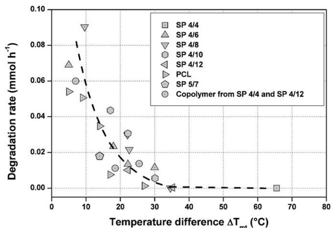
Fig. 4. Dependence of the degradation rate of aliphatic polyesters (SP refers to “saturated polyester”) from the difference between the degradation temperature and the melting temperature of the polyester ( $\Delta T_{mt}$ ). Degradation with lipase from *Pseudomonas* sp. at pH 7, monitored as cleavage of ester bonds [15].
