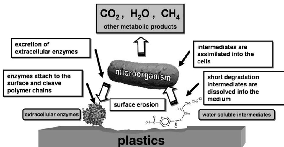
Fig. 1. Scheme of general mechanism of enzymatic catalyzed hydrolytic polymer degradation.
