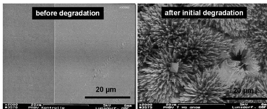
Fig. 2. Surface erosion at a PHBV-film incubated with an anaerobic microorganism (*Clostridium*, Strain 5a) on mineral salt agar for 7 weeks at 35 °C [5].
